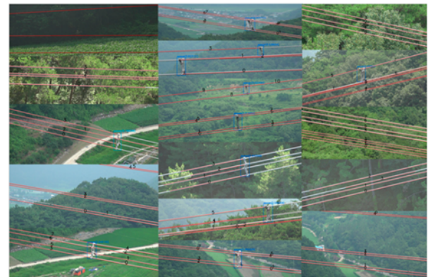
Figure 8. Power cord test findings. The suggested approach for detecting electricity lines is resilient to various lighting conditions and crowded backdrops. An ID number is written on the red-marked power cord that has been detected
