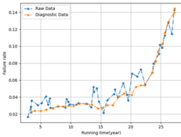
Figure 2. Transformer failure rate distribution curve
